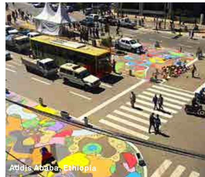
3. A multi-coloured ground artwork designed to improve pedestrian safety across the LeGare intersection in Addis Ababa.
